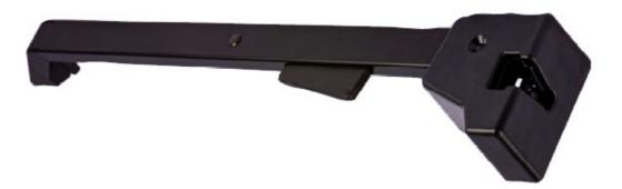
The compact 050-7120 10mm Single Rotor Latch with Handrail is designed for operator and compartment door applications for offhighway vehicles that require a remote interior release. The latch is incorporated into a rectangular tube for support for the opening and closing function of the door and provides for greater ease of operation (ergonomics) over direct releases.
